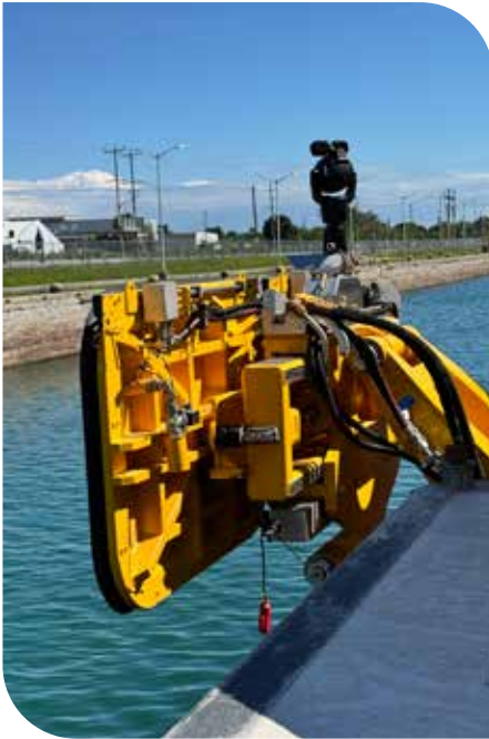
Close-up of a vacuum pad in the Hands-Free Mooring system.
